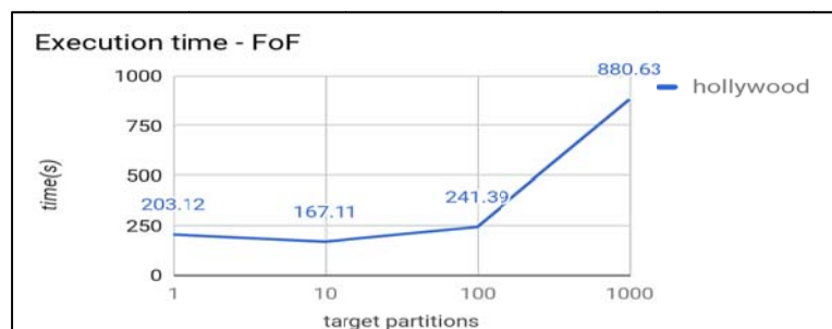
Fig. 15. Chart of the effect at runtime of dividing the problem into smaller
